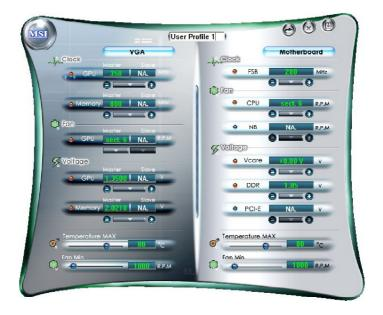
Use the draw bar to set the max system temperature. When the system temperature exceeds the threshold you defined, the system will pop up a warning message and shut down the system.
